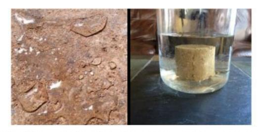
Laboratory testing revealed that the best performance is achieved at a mix ratio of 1 part **Soil Chem Road Material** to 1 part water and applied at a rate of .6 gallons per yard to a depth of 12". Following deep stabilization, the solution is sprayed topically at a rate of .2 gallons per yard and then compacted to a 90% compaction using a sheep foot and rollers.
